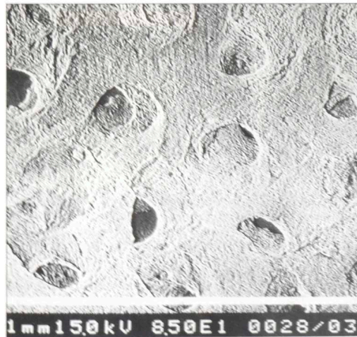
Fig. 2 Electron Microscopy of Porites Astreoides coral showing a regular system of interconnecting pores approximately 120 microns in diameter.
